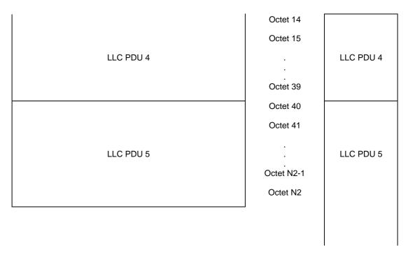
Figure B.8: Example for the case when a LLC PDU stretches over more than 2 consecutive in sequence RLC data blocks (LLC PDU 3 and LLC PDU 5).
