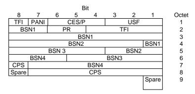
Figure 10.3a.3.9.1: Combined downlink RLC data block header for DBS-11 and DBS-12.
