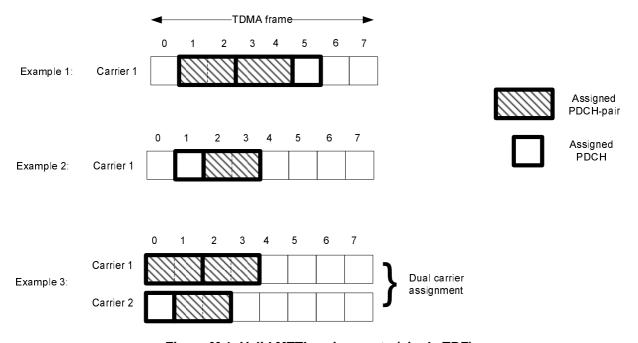
Figure M.1: Valid MTTI assignments (single TBF)
