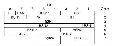
Figure 10.3a.3.8.1: Combined downlink RLC data block header for DBS-9 and DBS-10.
