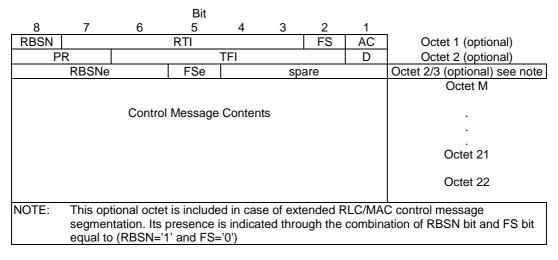
Figure 10.3.1.2: Downlink RLC/MAC control block message contents
