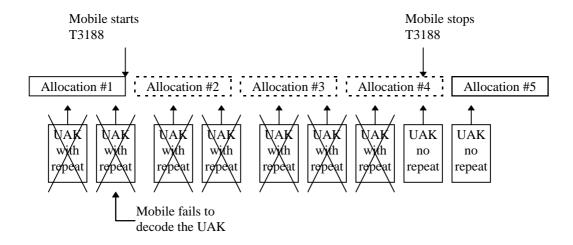
Figure E.3: Multiple Missed Uplink Ack/Nacks
