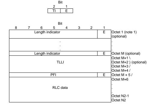
NOTE 1: If padding is used, then "Octet 1" shall be replaced by "Octet 7", see example in annex J.
