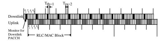
Figure D.9: Multislot Class 21 (Rx=6, Tx=4,Sum=NA), 4 timeslot uplink TBF
