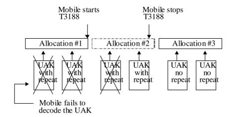
Figure E.2: Repeated Fixed Allocation with Missed ACK
