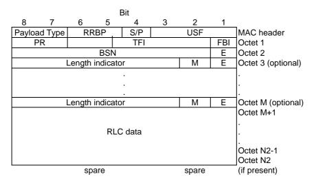
Figure 10.2.1.1: Downlink RLC data block with MAC header
