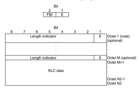
NOTE: If padding is used, then "Octet 1" shall be replaced by "Octet 7", see example in annex J.
