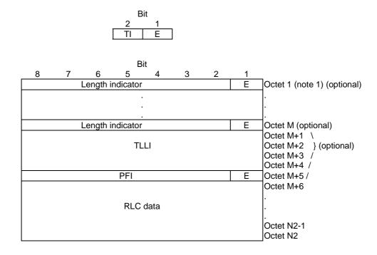
NOTE 1: If padding is used, then "Octet 1" shall be replaced by "Octet 7", see example in annex J.
