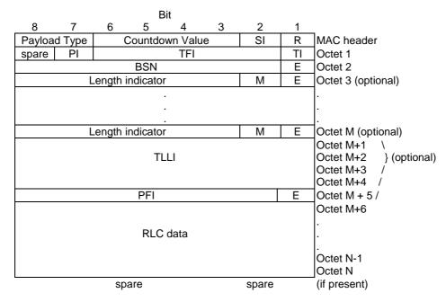
NOTE: The field mapping convention for GPRS (sub-clause 10.0b.3.1) applies. According to that, in particular regarding the TLLI field, the *most significant byte* of the TLLI value shall be mapped on octet M+1 and the *least significant byte* of the TLLI value shall be mapped on octet M+4 of the uplink RLC data block.
