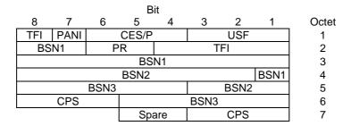
Figure 10.3a.3.5.1: Combined downlink RLC data block header for DAS-11 and DAS-12.
