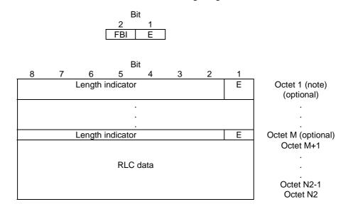
NOTE: If padding is used, then "Octet 1" shall be replaced by "Octet 7", see example in annex J.
