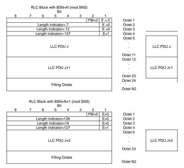
Figure B.11: Example for the case when the LLC PDU J+1 ends in the previous RLC data block and the start of the next LLC PDU J+2 is in the next RLC data block which is indicated using Ll=126 as the first LI in that RLC data block.
