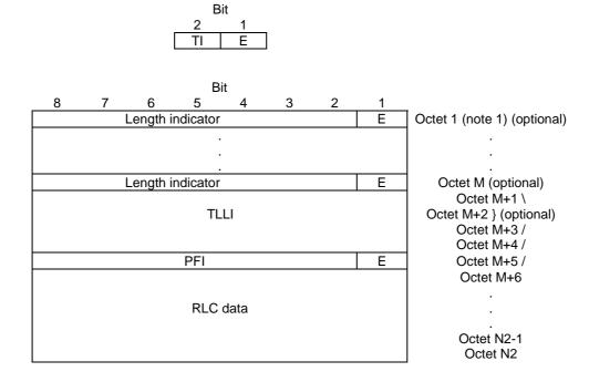
NOTE 1: If padding is used, then "Octet 1" shall be replaced by "Octet 7", see example in annex J.
