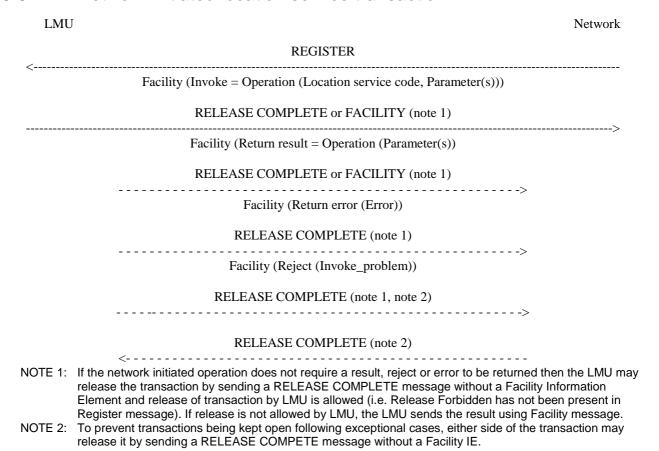
Figure 5.6.2: Network initiated location service transaction
