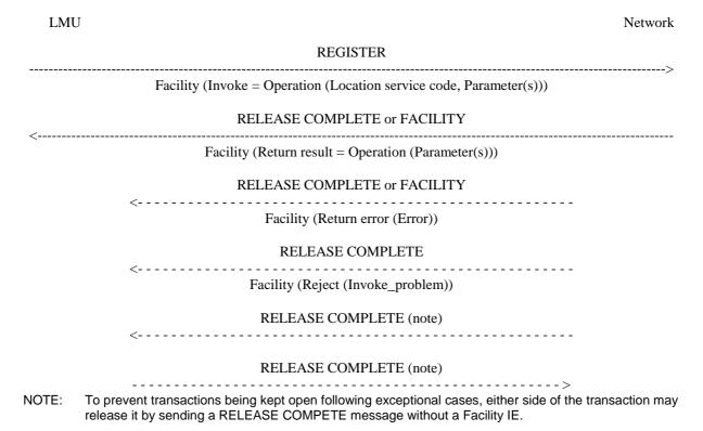
Figure 5.6.1: LMU initiated location service transaction
