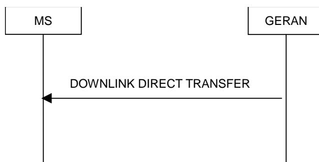
Figure 7.17.2.1: Downlink Direct transfer, normal flow
