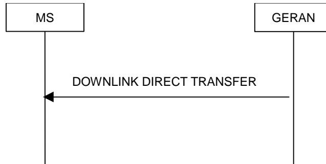
Figure 7.17.2.1/3GPP TS 44.118: Downlink Direct transfer, normal flow
