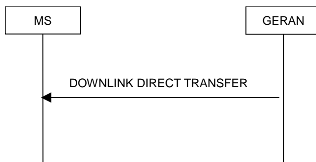
Figure 7.17.2.1/3GPP TS 44.118: Downlink Direct transfer, normal flow
