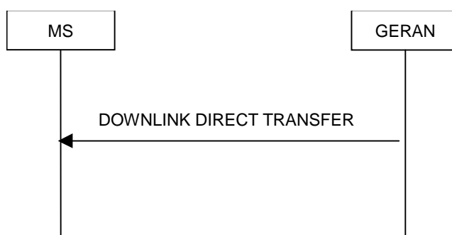
Figure 7.17.2.1/3GPP TS 44.118: Downlink Direct transfer, normal flow
