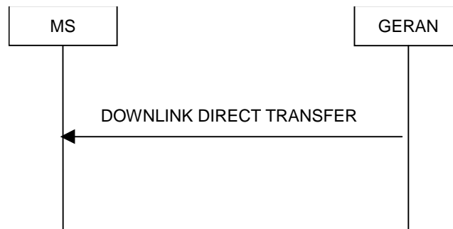
Figure 7.17.2.1: Downlink Direct transfer, normal flow
