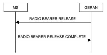
Figure 7.14.1.5: Radio Bearer Release, normal case
