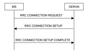
Figure 7.5.1.1: RRC Connection Establishment, network accepts RRC connection
