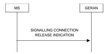
Figure 7.15.2.1.1: Signalling Connection Release Indication procedure, normal case
