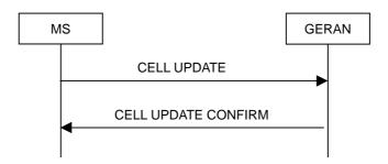
Figure 7.8.1.1: Cell Update procedure, basic flow
