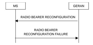
Figure 7.14.1.4: Radio Bearer Reconfiguration, failure case
