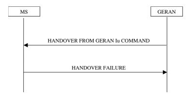
Figure 7.8.4.1.2: Inter-mode handover from GERAN lu mode, failure case
