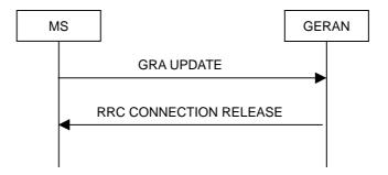
Figure 7.8.1.8: GRA Update procedure, failure case
