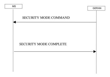
Figure 7.16.1.1: Security mode control procedure
