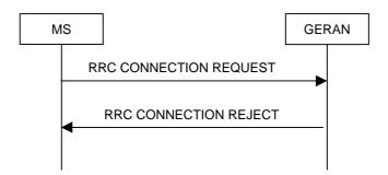
Figure 7.5.1.2: RRC Connection Establishment, network rejects RRC connection
