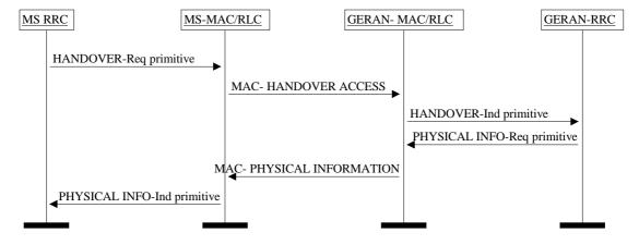
Figure 7.18.6.0.1: Handover Access procedure
