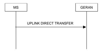
Figure 7.17.3.1: Uplink Direct transfer, normal flow
