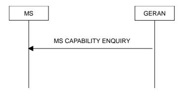
Figure 7.7.1.1: MS Capability Enquiry procedure, normal flow
