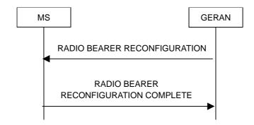
Figure 7.14.1.3: Radio Bearer Reconfiguration, normal flow
