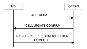
Figure 7.8.1.4: Cell Update procedure with radio bearer reconfiguration
