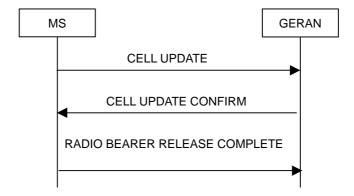
Figure 7.8.1.3: Cell Update procedure with radio bearer release
