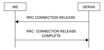
Figure 7.5.2.1: RRC Connection Release procedure
