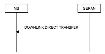
Figure 7.17.2.1: Downlink Direct transfer, normal flow
