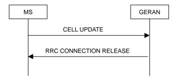
Figure 7.8.1.5: Cell Update procedure, failure case
