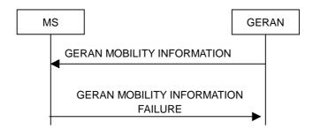
Figure 7.8.3.2: GERAN Mobility Information procedure, failure case
