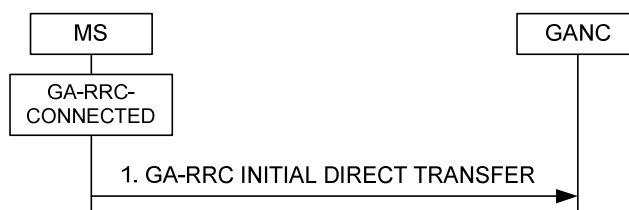
Figure 8a.2.1.1 Initial direct transfer, normal flow
