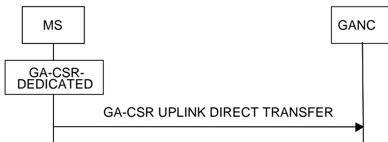
Figure 7.2.1.1 Uplink Direct Transfer, normal flow
