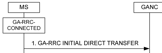
Figure 8a.2.1.1 Initial direct transfer, normal flow
