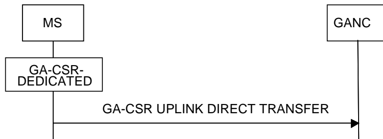
Figure 7.2.1.1 Uplink Direct Transfer, normal flow
