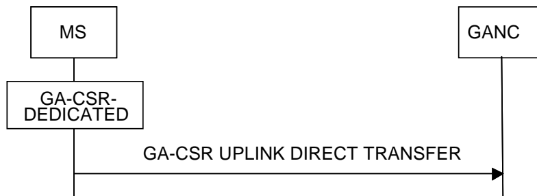
Figure 7.2.1.1 Uplink Direct Transfer, normal flow
