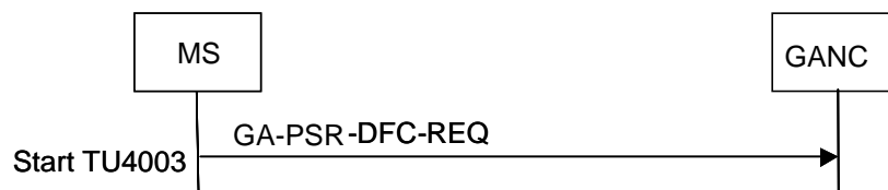
Figure 8.11.1 MS initiated Downlink Flow Control
