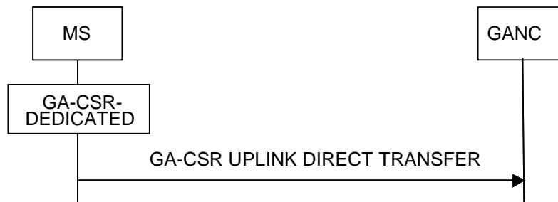
Figure 7.2.1.1 Uplink Direct Transfer, normal flow
