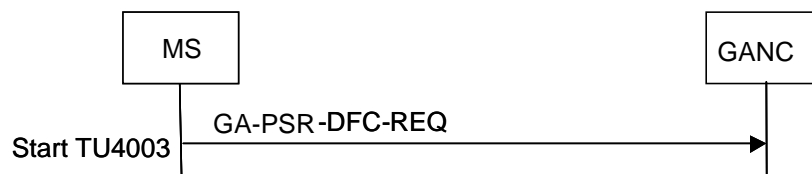
Figure 8.11.1 MS initiated Downlink Flow Control
