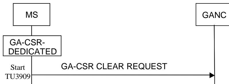
Figure 7.5.1.1 Initiation of GA-CSR connection release by MS
