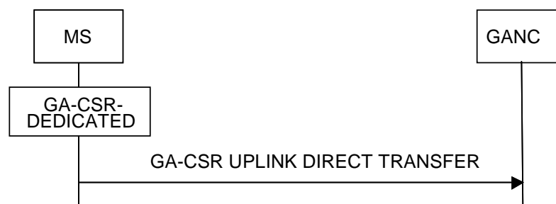
Figure 7.2.1.1 Uplink Direct Transfer, normal flow
