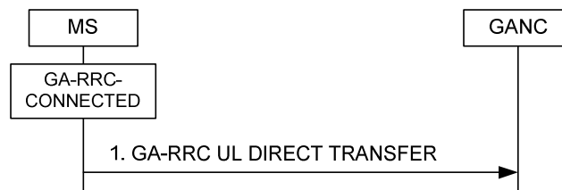
Figure 8a.2.3.1 Uplink direct transfer, normal flow
