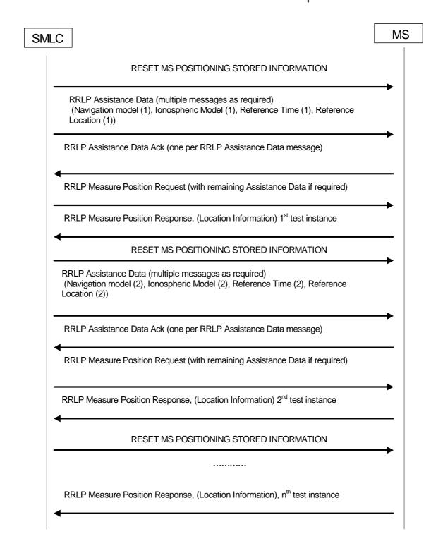
Figure M.5.1: MS-Based A-GPS Message Sequence
