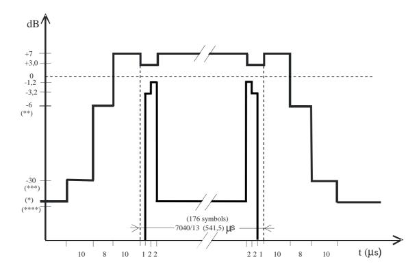
Figure B.9: Time mask for higher symbol rate bursts (HB) at 16-QAM and 32-QAM modulation with wide pulse shaping filter
