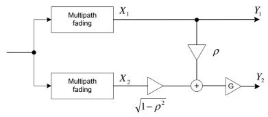
Figure N.2.1: Single input - dual output channel model for MS Receiver Diversity - DARP ph II
