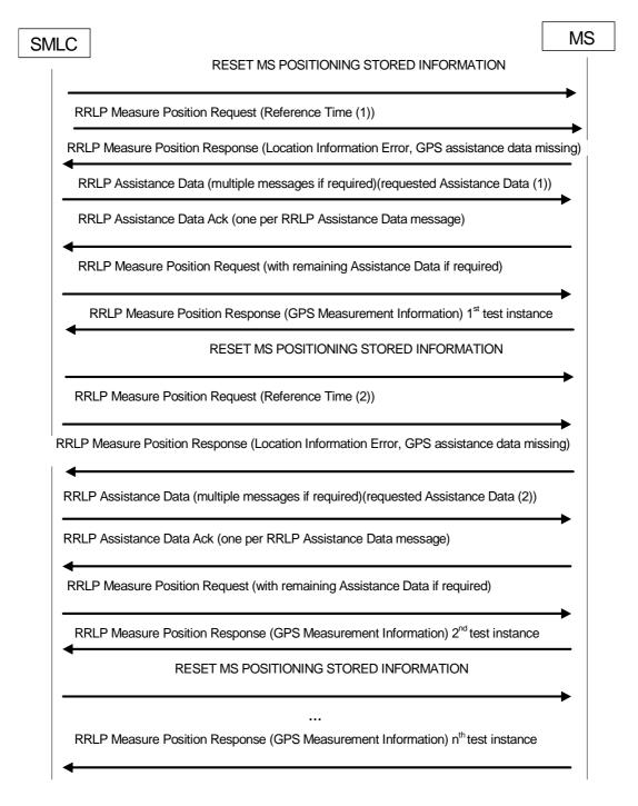
Figure M.5.2: MS-Assisted A-GPS Message Sequence
