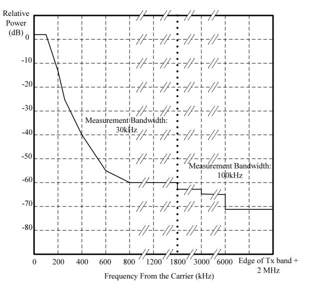
Figure A.3c: DCS 1 800 and PCS 1900 MS spectrum due to QPSK, 16-QAM and 32-QAM modulation with higher symbol rate using using wide pulse shaping filter
