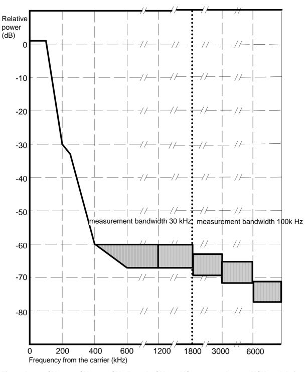
Figure A.1a: GSM 400, GSM 900, GSM 850 and GSM 700 MS spectrum due to GMSK modulation
