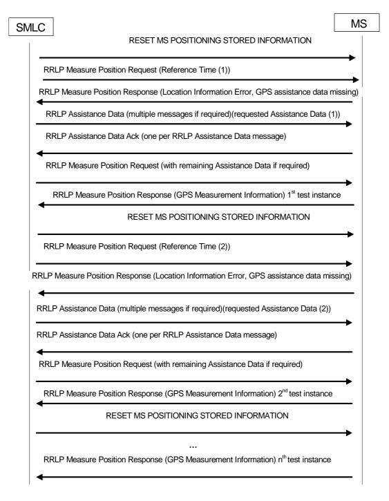
Figure M.5-2: MS-Assisted A-GPS Message Sequence
