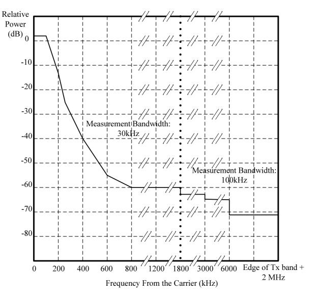
Figure A.1c: GSM 400, GSM 900, GSM 850 and GSM 700 MS spectrum due to QPSK, 16- QAM and 32-QAM modulation with higher symbol rate using wide pulse shaping filter
