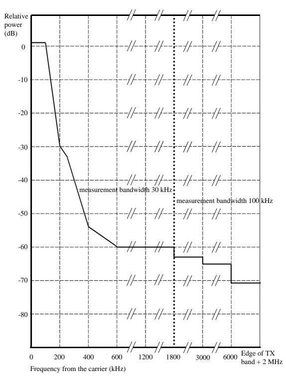
Figure A.1b: GSM 400, GSM 900, GSM 850 and GSM 700 MS spectrum due to 8-PSK and 16-QAM modulation with normal symbol rate and QPSK, 16-QAM and 32-QAM modulation with higher symbol rate using narrow BW pulse shaping filter
