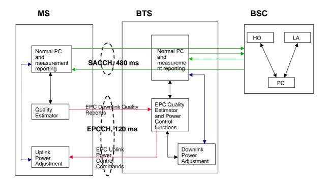
The BSC has the control over which power control loop is in use. For the uplink power control, this is signalled with one control bit on the Abis interface to the BTS, which in turn informs the MS, when the enhanced power control shall be used.
