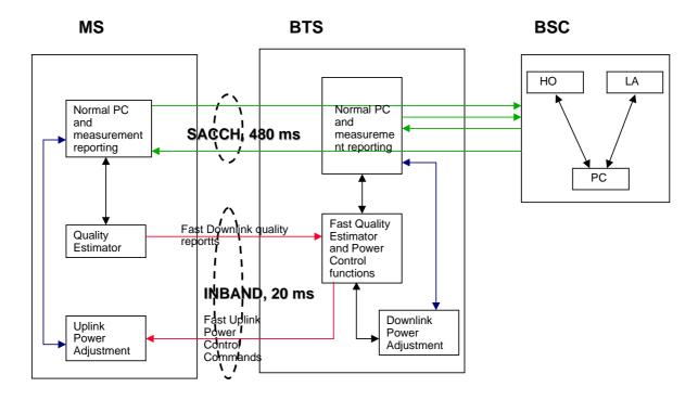
The BSC has the control over which power control loop is in use. This is signalled with one control bit on the Abis interface to the BTS, which in turn informs the MS, when the fast power control loop shall be used. When FPC is not activated, there is no requirement for either the BTS nor the MS to perform quality estimations or sending commands/reports via E-IACCH.
