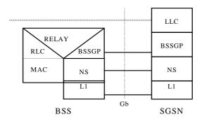
Figure 4.1: BSSGP's position within the Gb-interface protocol stack
