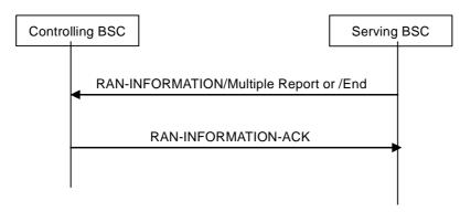
Fig 8c.2.3: Acknowledged RAN Information Send procedure
