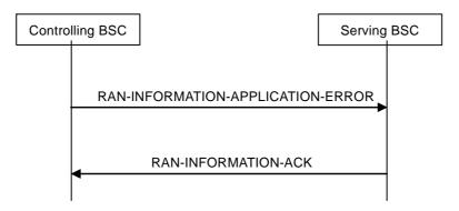
Fig 8c.2.4: RAN Information Application Error procedure
