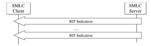
In the autonomous mode the procedure consists of one or more RIT Indication operations.
