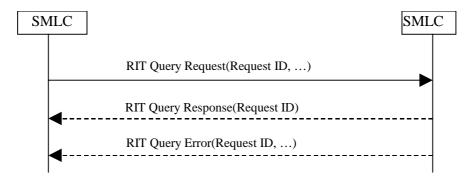
This operation allows a SMLC to query RIT information from another SMLC. This operation consists of sending of a RIT Query Request. It includes the Request ID , that is used to identify different queries. The RIT Query Request also includes the description of the scheduling of RIT Indication operations in the reverse direction. This includes the following cases:
