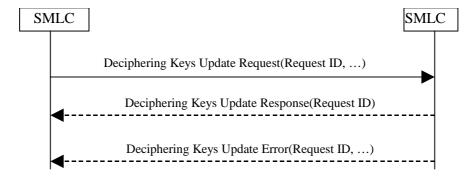
This operation allows a SMLC controlling deciphering keys to send the keys to another SMLC Client.
