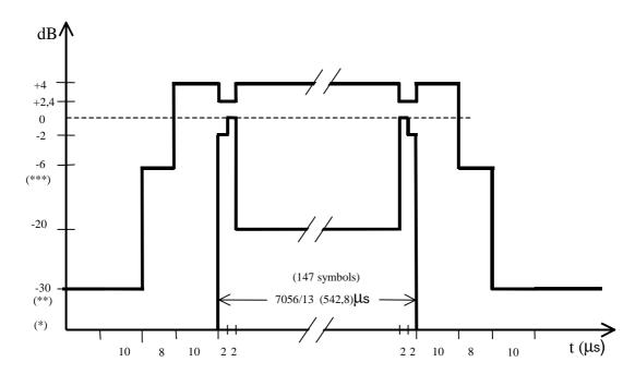
NOTE: The 0 dB reference is equal to the power Pmax or Pmin.
