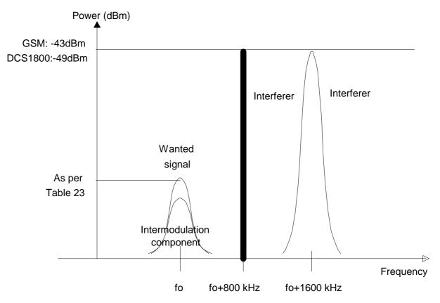
Figure 6: Example of RX intermodulation rejection
