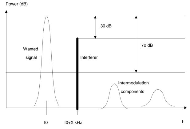
Figure 5: Example of TX intermodulation attenuation
