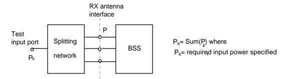
Figure 1a: Receiver test setup
