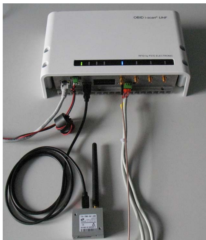
Figure A.5: Modified Feig OBID i—scan® UHF reader (top) with Triorail GSM-R receiver (bottom)
