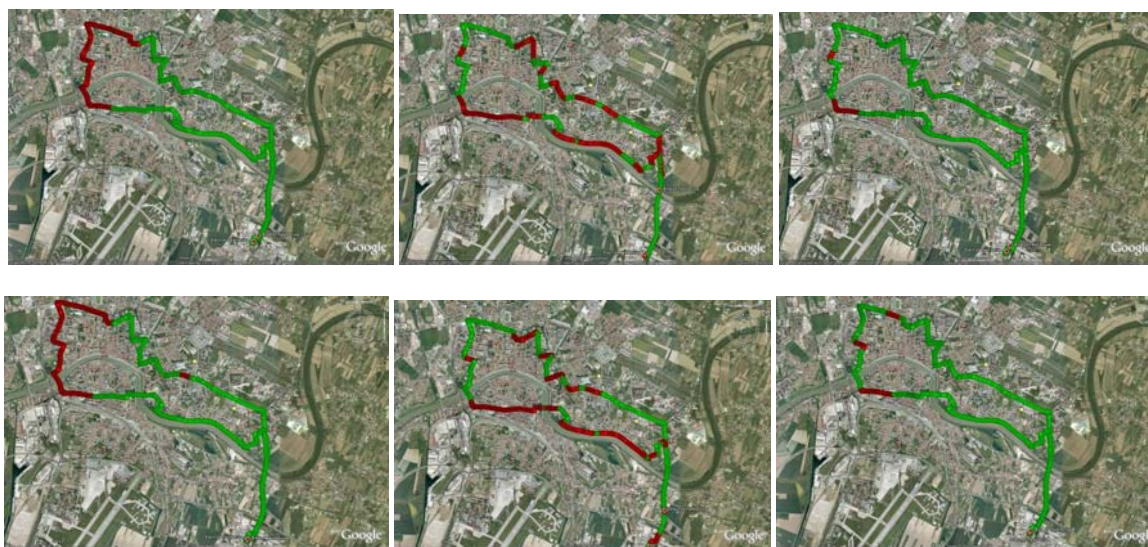
Figure 7.50: Service availability vs. location, class 1 configuration Terrestrial only (left), Satellite only (mid), code combining (right) Red spots identify areas in which the ESR5(20) criterion is not fulfilled Receiver 1 (top) and 2 (bottom)
