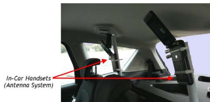
Figure A.13.47: In-car receivers
