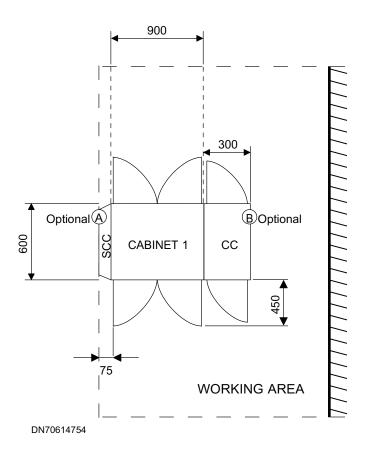
A = Optional side cable conduit (SCC) is connected to either side of the BSCC in an equipment room with a raised floor. The SCC is not used when overhead cabling or the cabling cabinet is in use.
