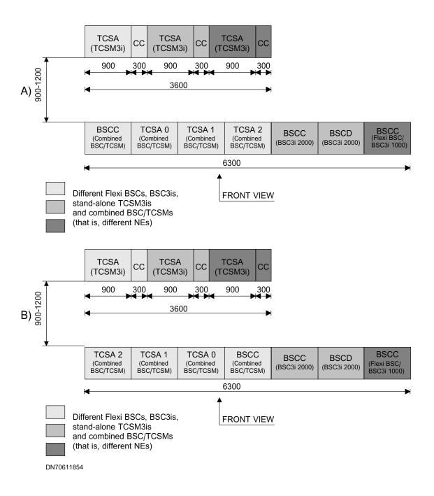
Figure 3. Equipment room without raised floor, an example
