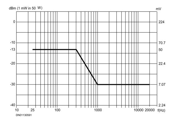
Figure 7. Maximum level of narrowband noise for the DX 200 network elements
