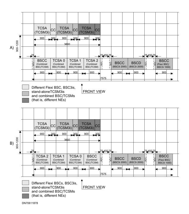
Figure 5. Equipment room with raised floor, example 2
