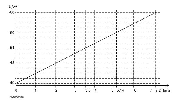
Figure 8. Hold-up time per input voltage
