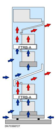
Figure 9. Ventilation in the equipment room, a TCSM3i cabinet as an example
