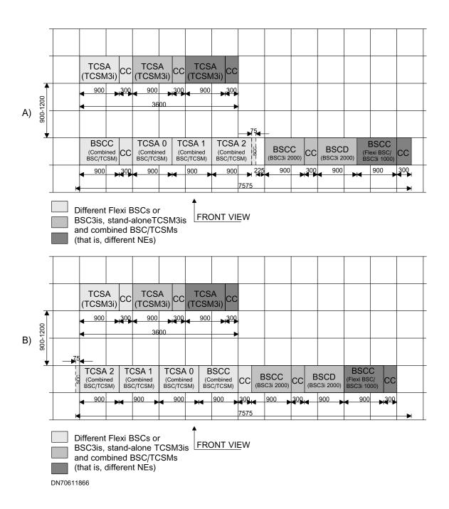
Figure 4. Equipment room with raised floor, example 1
