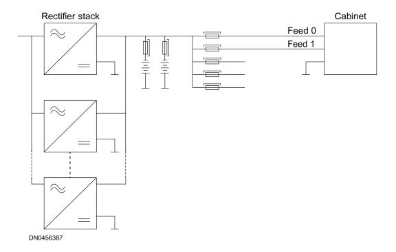
Figure 6. N+1 rectifier system with two separate backup battery strings
