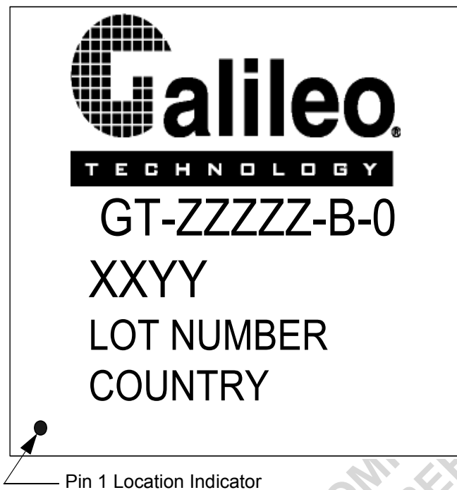
Figure 92: Package Markings and Pin 1 Location
