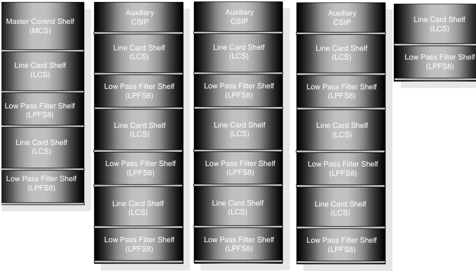
Figure 1-1: Config. A: Data Plus Voice, LPFS8 Co-Located
