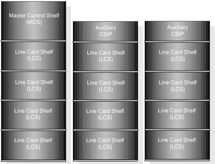
Figure 1-14: D50 with 12 LCSs and 2 Auxiliary CSIPs (Data Only)
